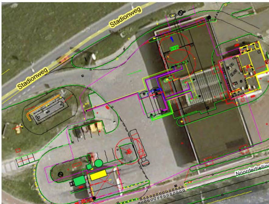
Figure 3: Virtual Hydrogen Refueling Station, projected on the existing refueling station; Hydrogen installations in green and yellow in the lower left corner
