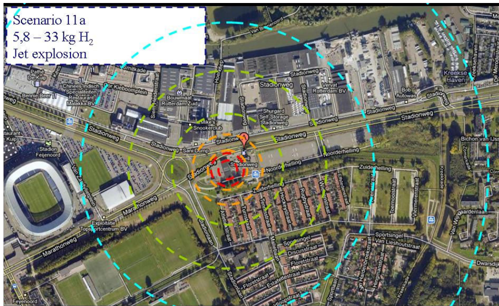
Figure 10: Side-on overpressure levels of the blast from a worst case exploding hydrogen jet for scenario 11a (red – 30 kPa, orange – 10 kPa, green – 3 kPa, blue – 1 kPa)
