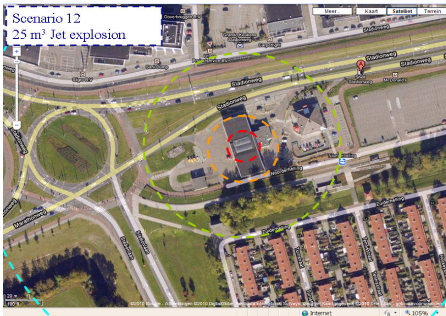
Figure 13: Side-on overpressure levels of the blast from a worst case exploding hydrogen jet for scenario 12 (red – 30 kPa, orange – 10 kPa, green – 3 kPa, blue – 1 kPa)
